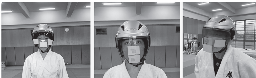
図1b フルフェイスヘルメットに感水紙を貼付（左：外側の感水紙位置、中央：内側の感水紙位置、右：実施時の装着の様子） Fig. 1b Water-sensitive paper attached to a full-face helmet (Left: position of water-sensitive paper on the outside, Center: position of water-sensitive paper on the inside, Right: view of attachment during implementation)
